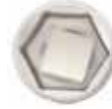
NPP drives the bolt on the sides and not on the corners
